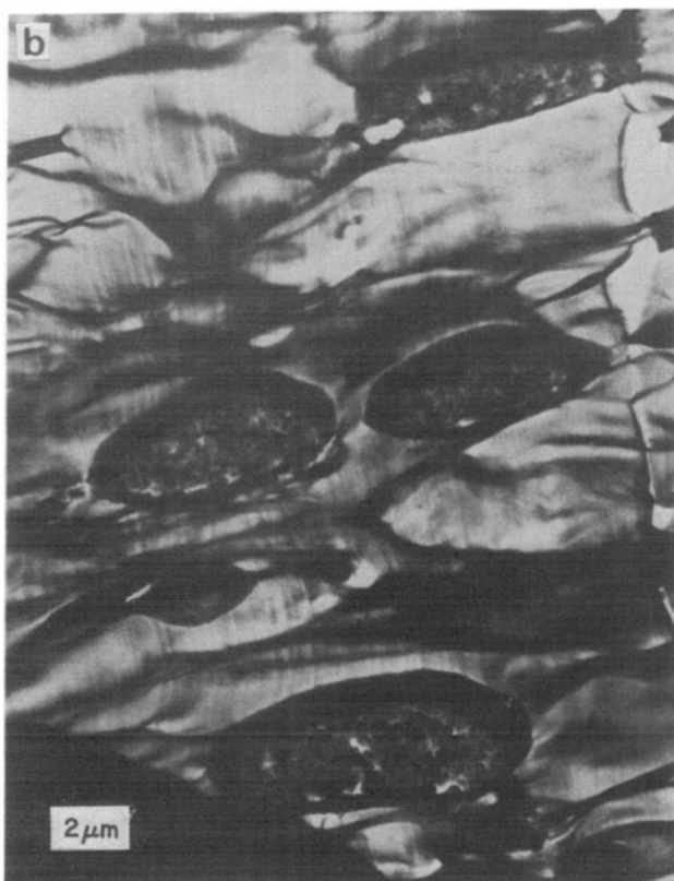
Figure 10(b) Transmission electron micrograph of 60 mole% PHB copolyester compression moulded at 285°C
